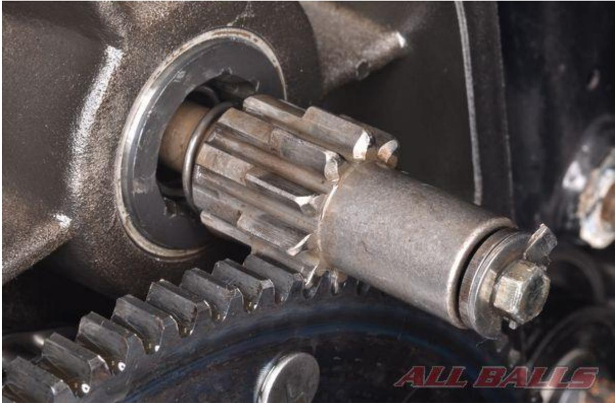
Extend the pinion gear so it can be held by the clutch driven gear and loosen the jack shaft bolt. Wrap the pinion gear with a rag and hold it with pliers if needed to keep it from turning when the bolt is loosened.
