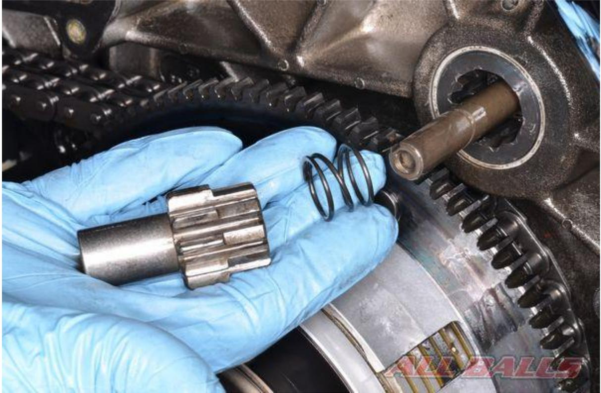
Remove the pinion gear and spring, and check for any damaged teeth on the starter driven gear on the clutch basket. Replace the components as necessary.
