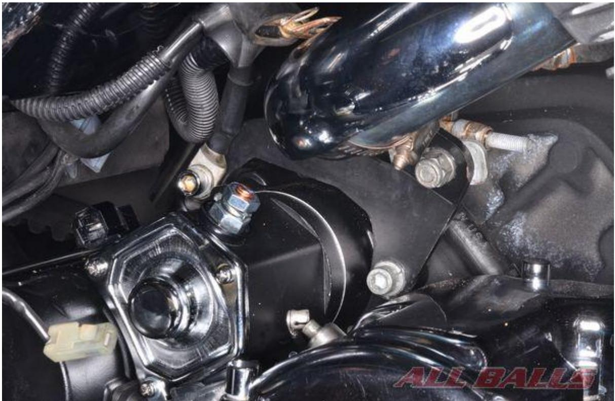
Remove the 2 starter motor mounting bolts. Some models may require the removal of an exhaust bracket.
