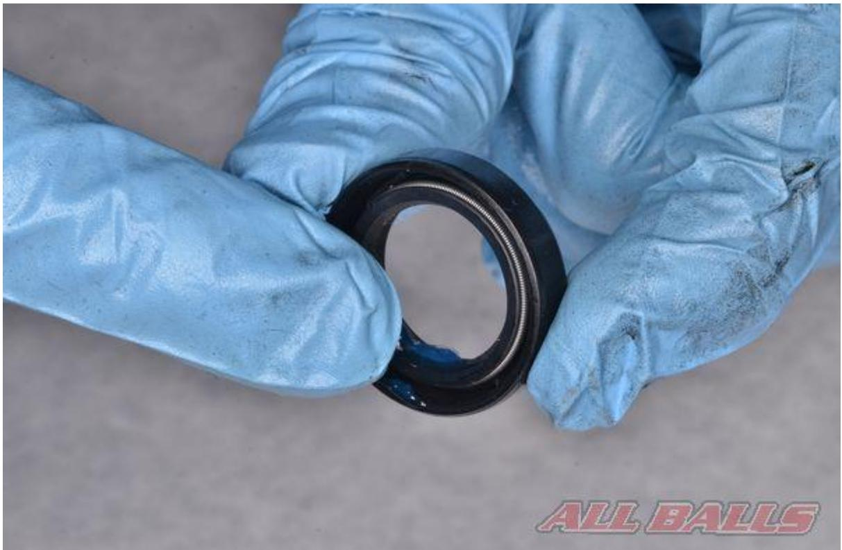
Apply a thin coat of grease to the new oil seal lips.
