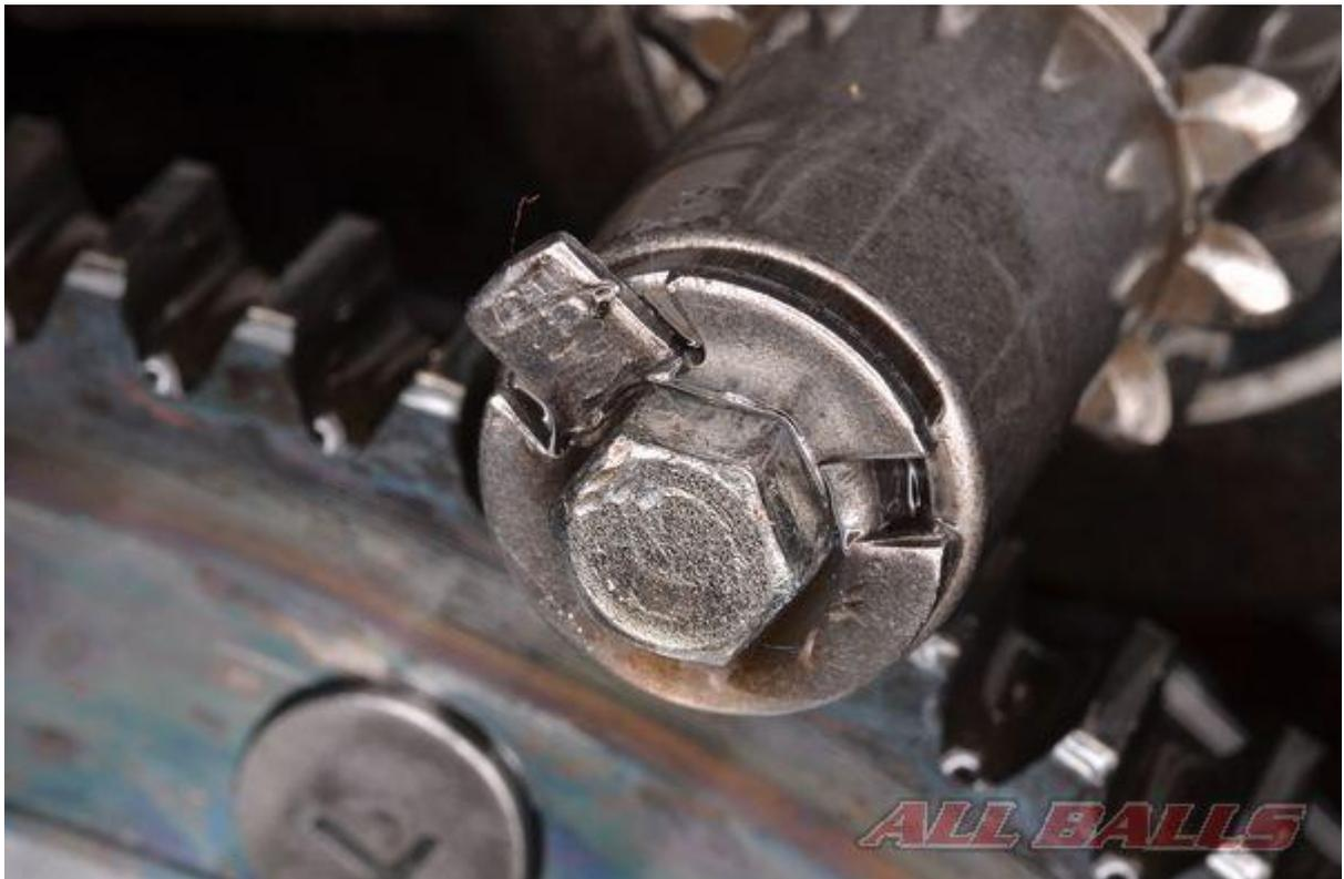
Bend the tab on the lock washer.
