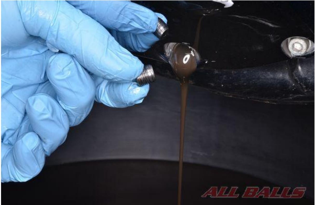
Remove the drain plug and allow the primary oil to drain completely.
