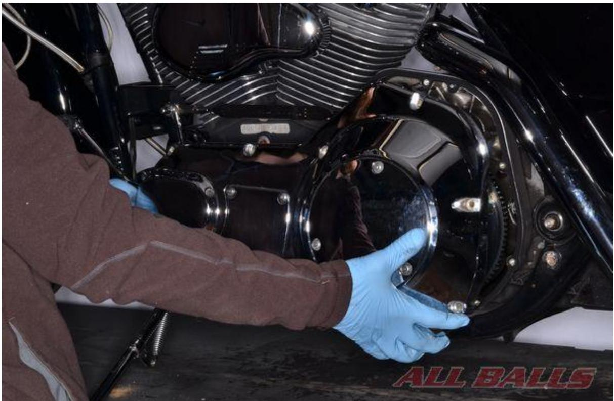
Remove the mounting bolts and the primary chain case cover.
