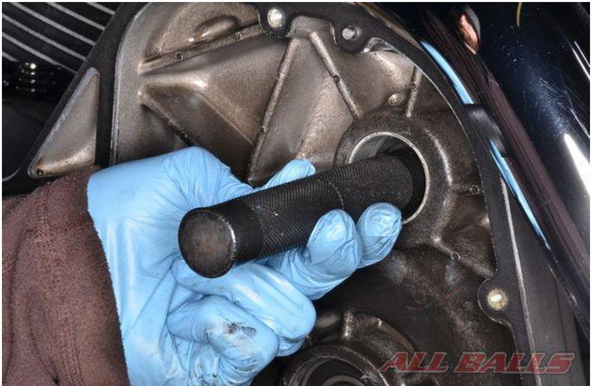
Install the new jack shaft oil seal into the left case half until it is fully seated.
