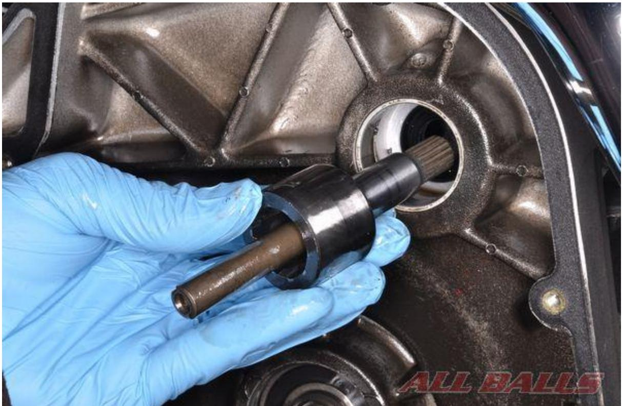
Remove the coupling and the old jack shaft.
