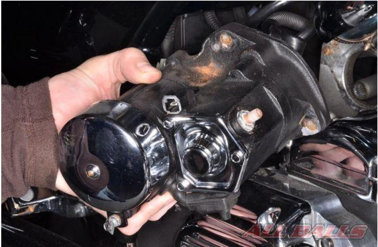
Remove the starter motor.
