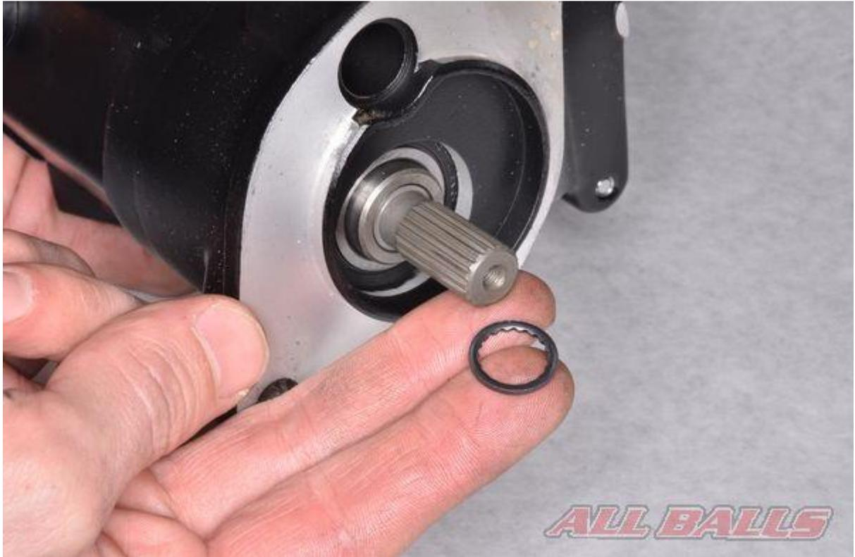
Install the the splined washer onto the new starter motor, a small dab of grease will help hold it in place. Apply a thin coat of grease to the starter motor splines.
