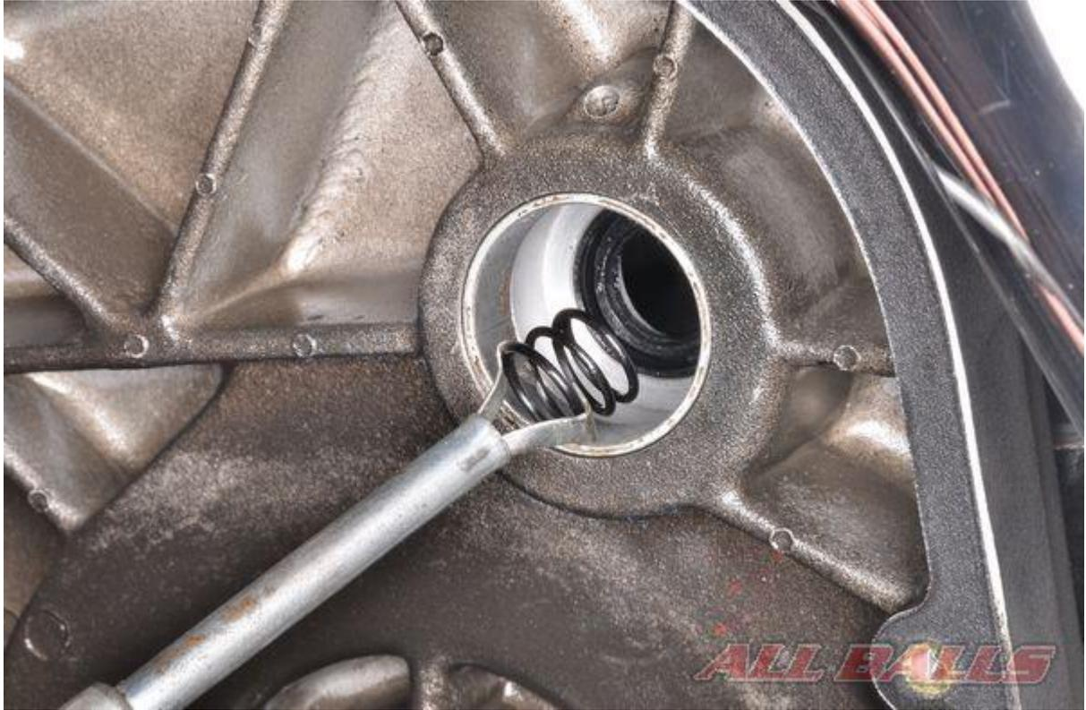
Using a suitable holding tool, carefully place the spring onto the starter motor shaft. Avoid damaging the oil seal or dropping the spring.
