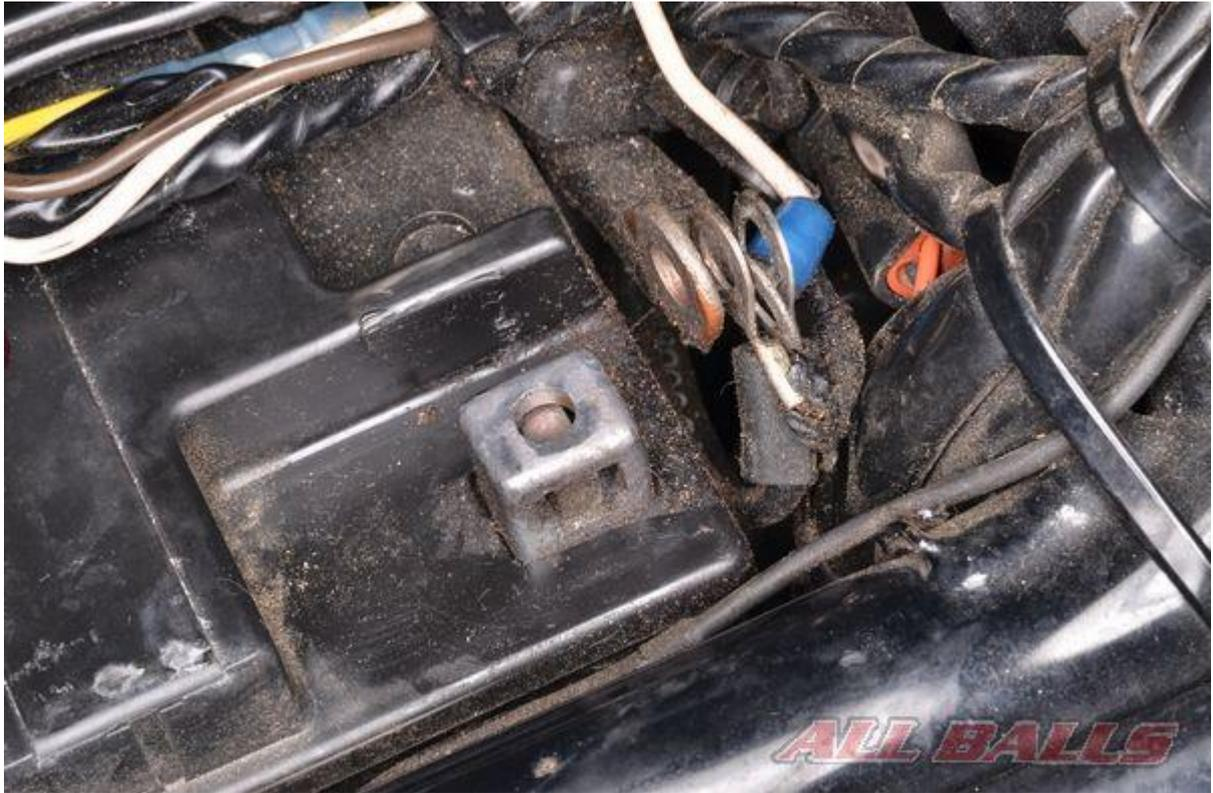
Disconnect the ground lead from the battery.
