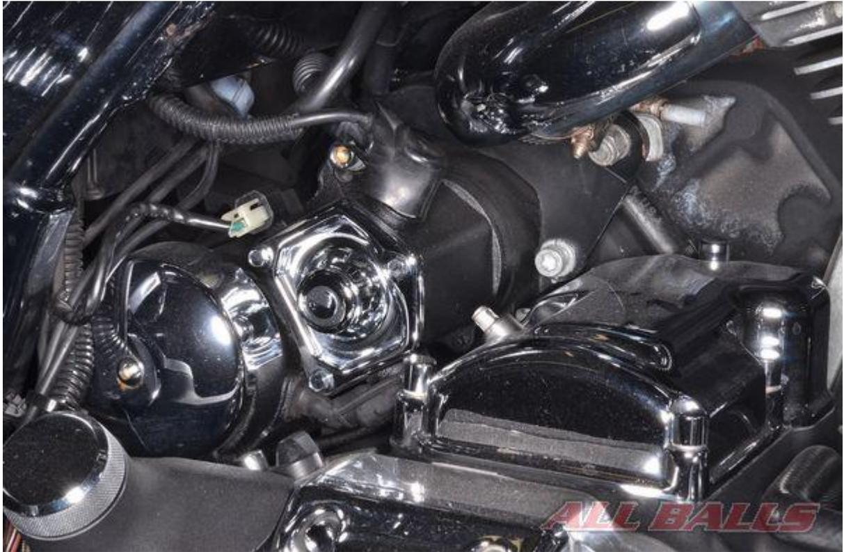
Connect the solenoid lead and battery cables, pull the rubber boot over the cables.
