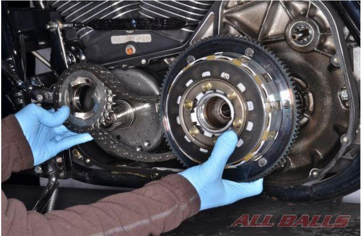
Follow the manufacturers instructions and remove the clutch and primary chain as an assembly.
