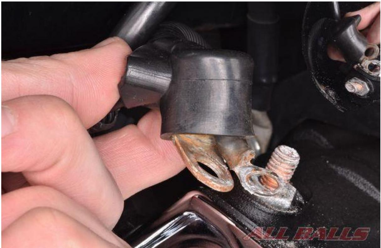
Pull back the rubber boot, remove the lock nut and free the starter motor cables.
