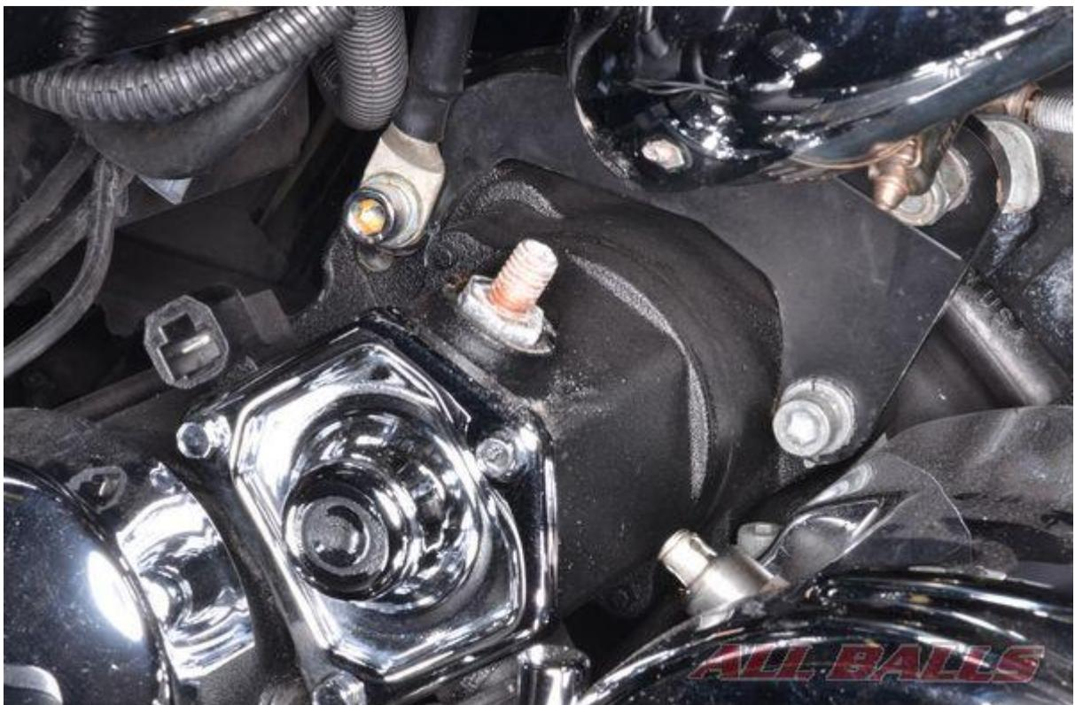
Install the new starter motor onto the engine. Tighten the bolts to specification with a torque wrench.
