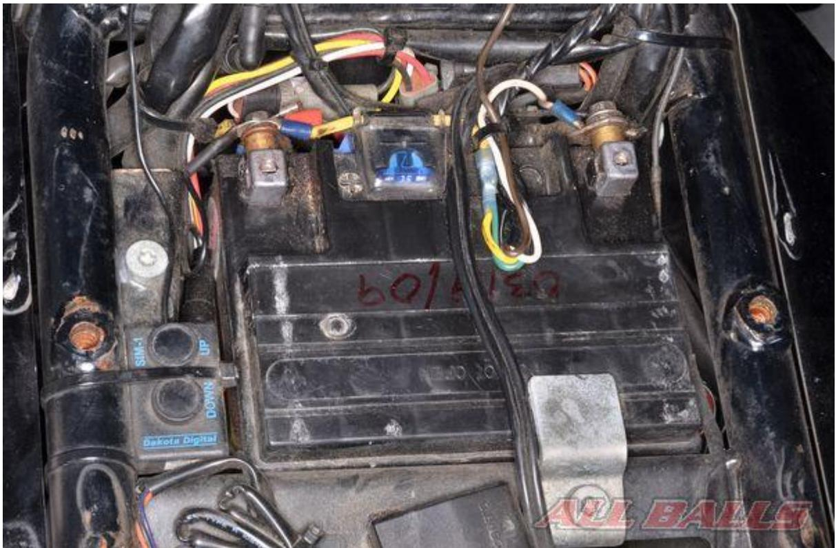
Connect the negative battery lead.
