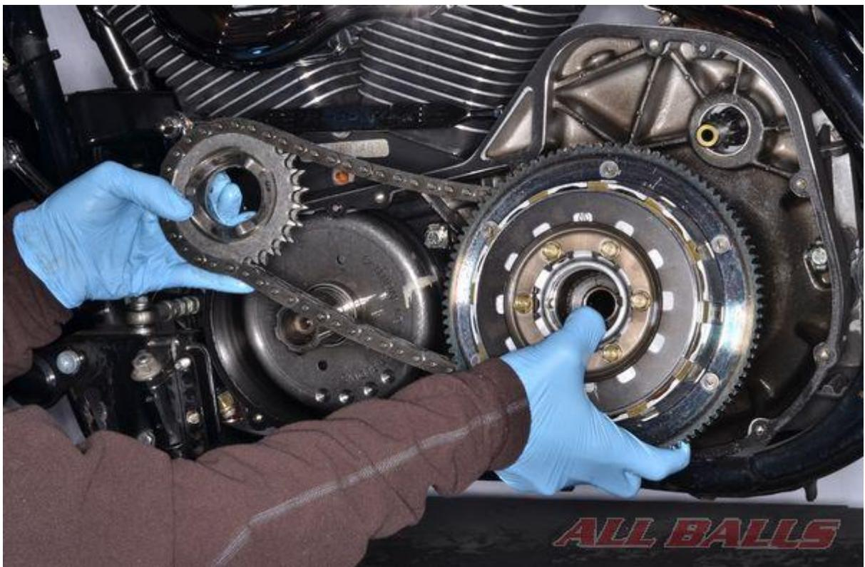
Install the clutch and primary assembly, follow the manufacturers instructions for proper reassembly.
