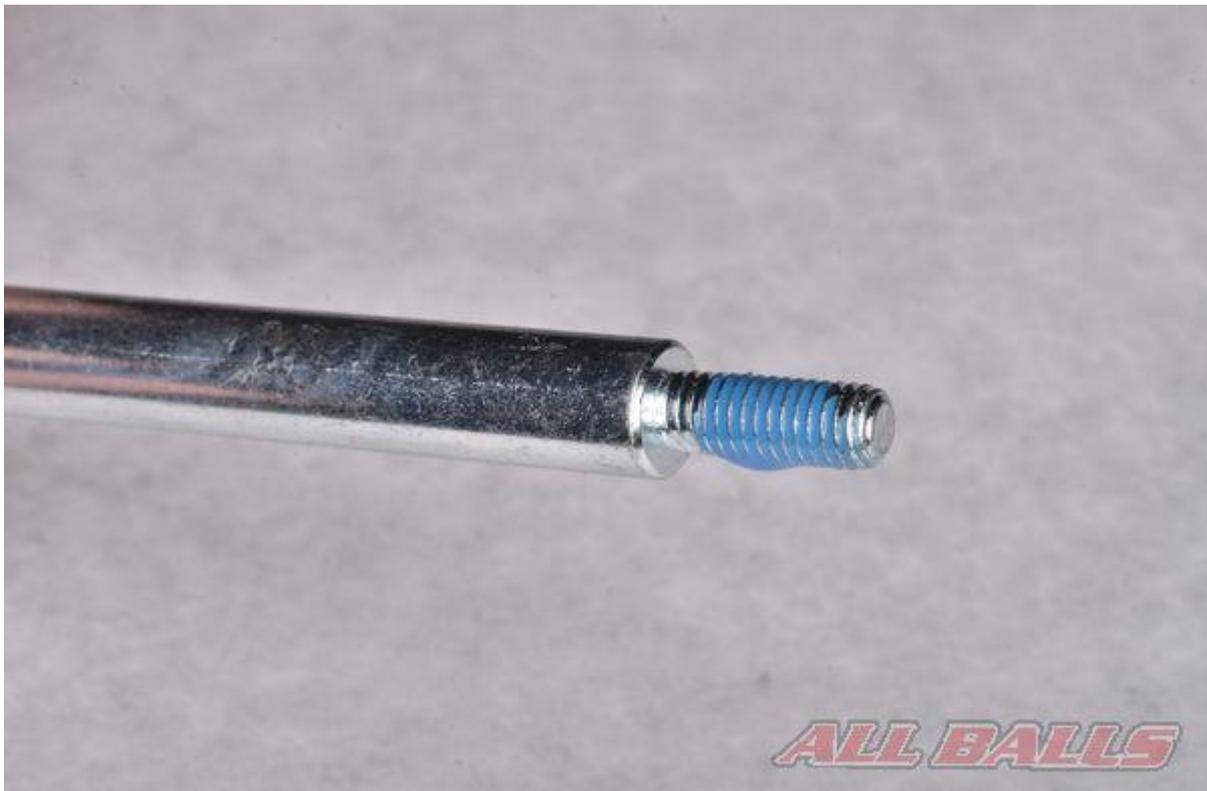
Apply non-permanent thread locking agent to the bolt threads.
