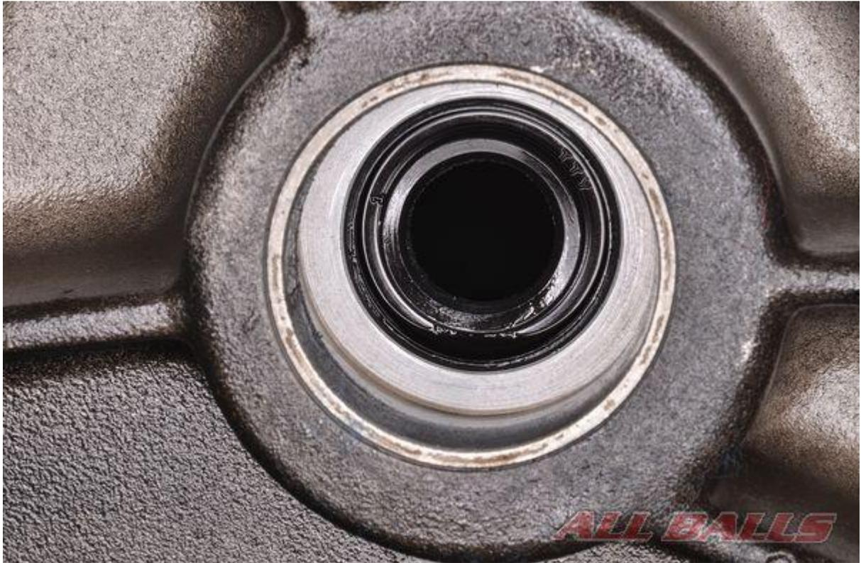
Drive out the old jack shaft oil seal and note the direction of the seal for installation.
