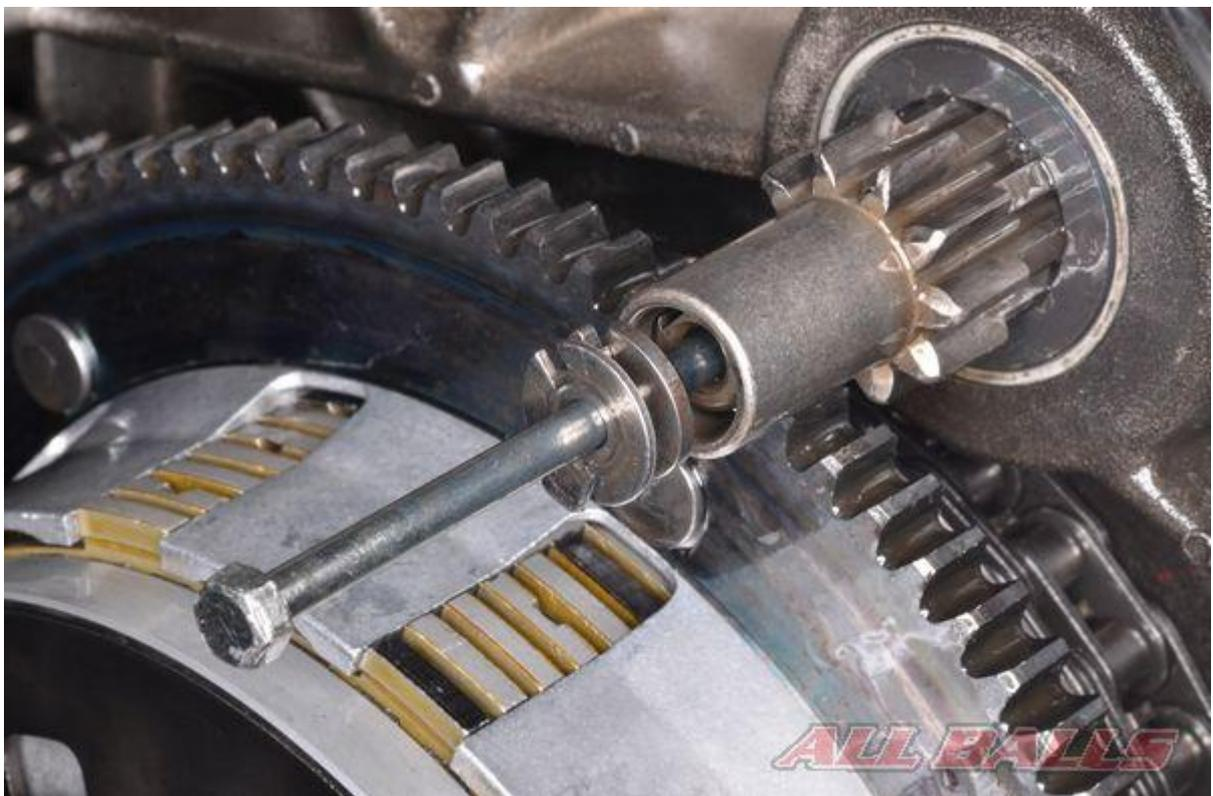
Remove the jack shaft bolt and washers.
