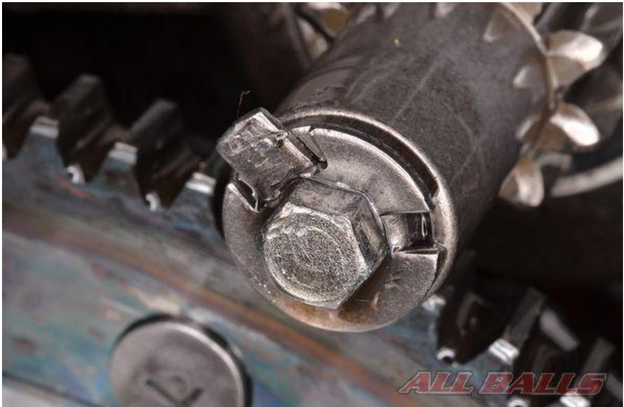
Bend the tab on the lock washer.
