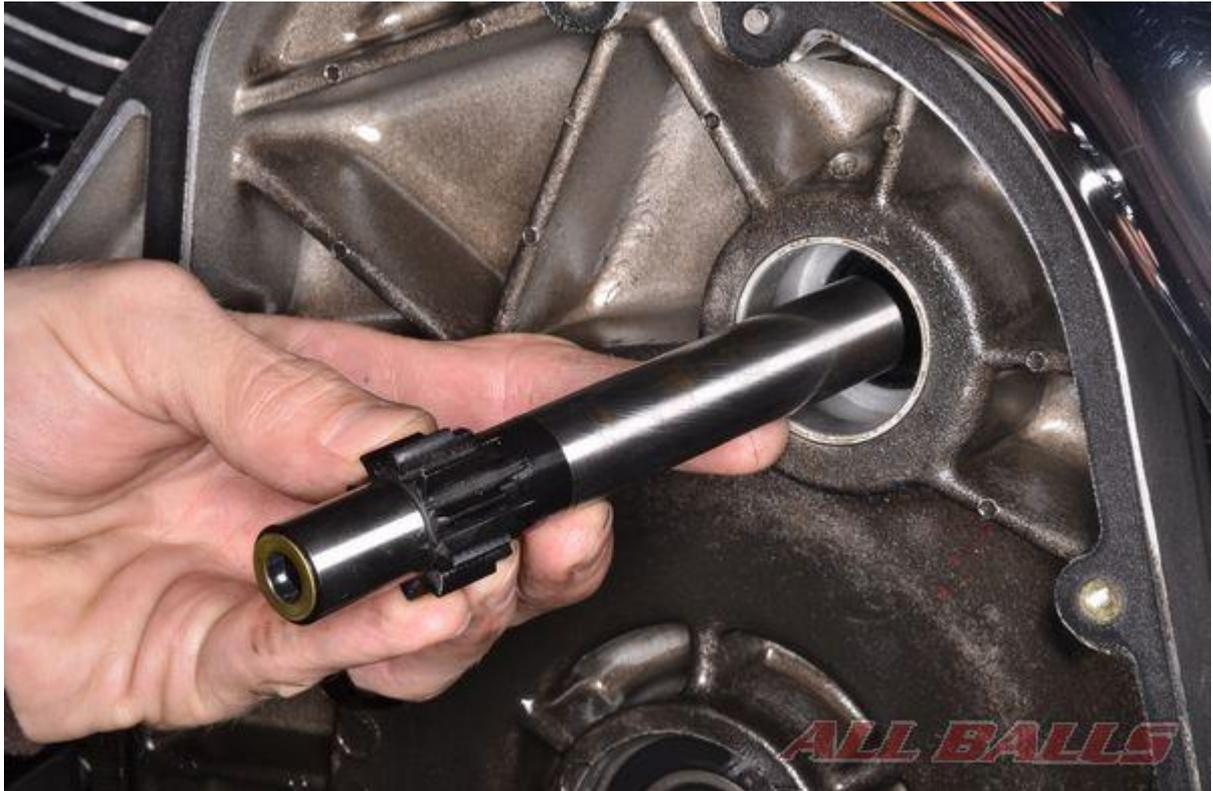
Install the new jack shaft onto the starter motor shaft, carefully guide it through the oil seal. Make sure it fits correctly- you will feel it press against the spring.
