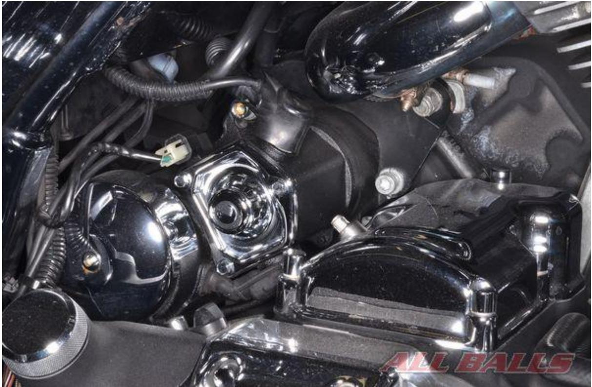
Locate the starter motor on the right side of the machine.
