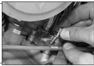
**STEP 5:** After removing the OEM oil pressure switch from the engine case, clean it, apply teflon thread sealant paste or teflon tape to its threads and screw it into the adaptor as shown. Apply thread sealer or tape to the threads of the adaptor as well and thread it into the engine case ensuring the threaded hole is pointing straight up.
