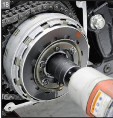
Remove the clutch hub nut (left-hand threads).
