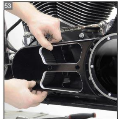
53 Install the front pulley cover onto the standoffs.
