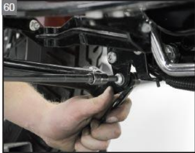
60 Install and tighten the engine guard mounting bolt.
