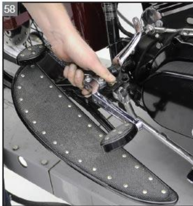
Align the footboard and shifter assembly with the frame.
