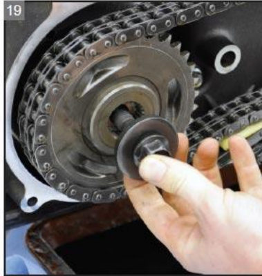
Remove the compensator bolt.
