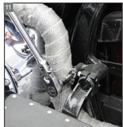
11 Remove the front exhaust hanger's mounting hardware.
