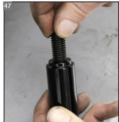
47 Thread the set screw into the standoffs.
