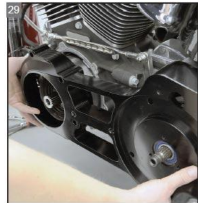
Install the motor plate onto the mainshaft.
