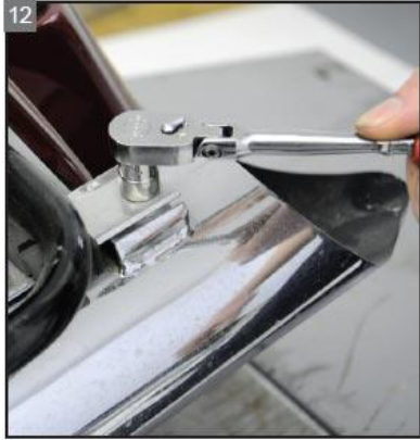
12 Loosen and remove the muffer hanger's mounting hardware.
