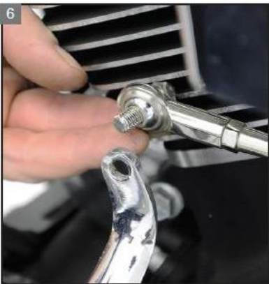
6 Remove the shift linkage from the front shift arm.
