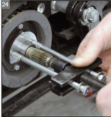
Slide the inner primary bearing race tool onto the race.
