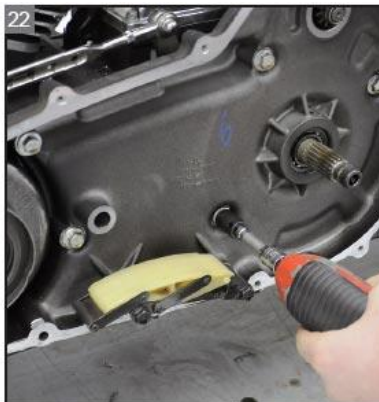
Remove the inner primary mounting bolts.
