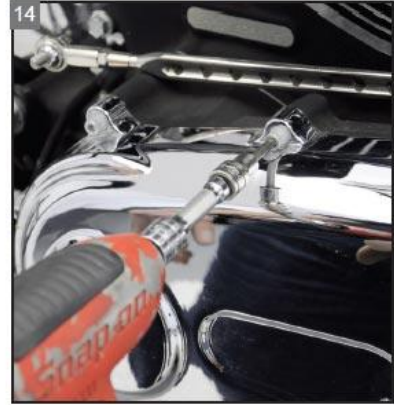
14 Remove the outer primary mounting hardware.
