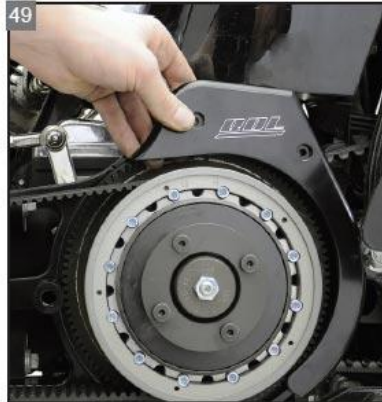
49 Install the starter cover onto the motor plate.
