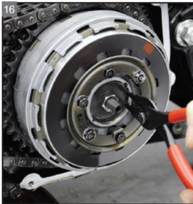
16 Remove the clutch adjuster plate Snap ring.
