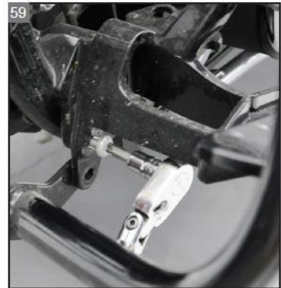
Install the footboard bracket mounting bolts.
