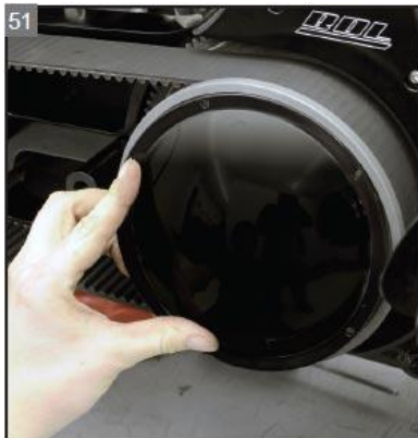
51 Install the clutch cover onto the clutch basket.
