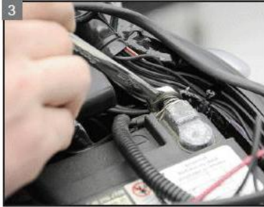
3 Disconnect the negative battery cable.
