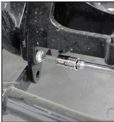
7 Remove the engine guard hardware and the three footboard mounting bolts.
