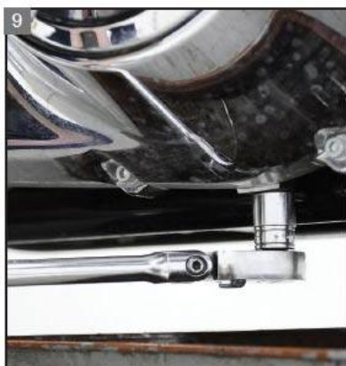
9 Remove the primary drain plug.
