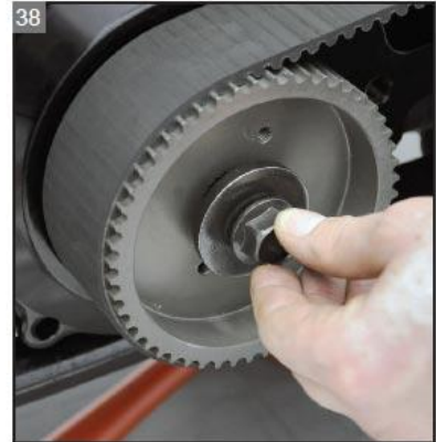
Install and torque the front pulley bolt.
