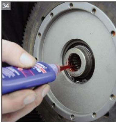
34 Apply red Threadlocker to the clutch hub splines.
