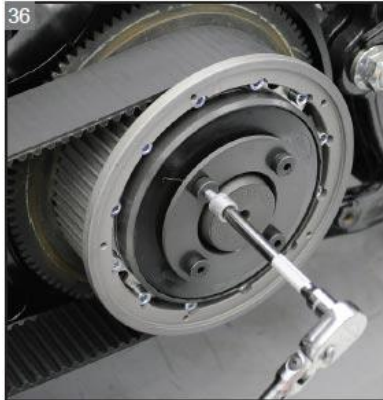
Remove the pressure plate mounting hardware.
