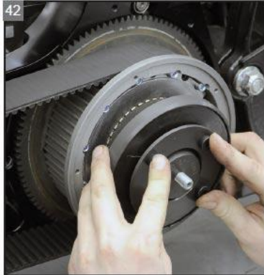
42 Install the pressure plate onto the clutch hub.
