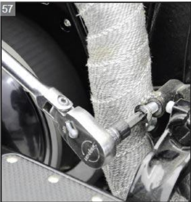
Install the exhaust's front mounting hardware.
