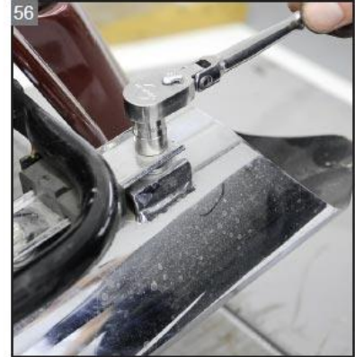
Install and tighten the muffler hanger hardware.
