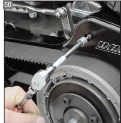
50 Install and tighten the starter cover mounting hardware.
