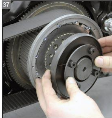
Remove the pressure plate.
