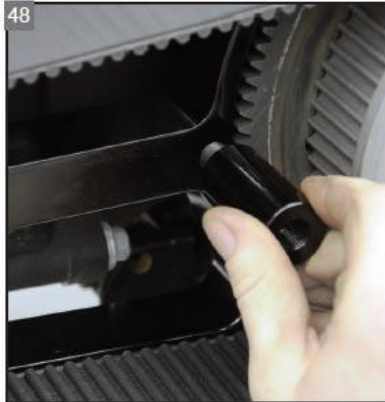
48 Install the standoffs into the motor plate. The relieved standoff goes in the rear, facing the motor plate.
