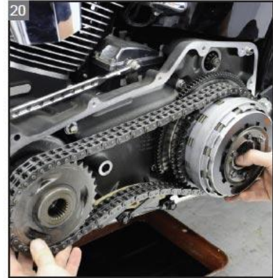
Remove the clutch and compensator assembly.
