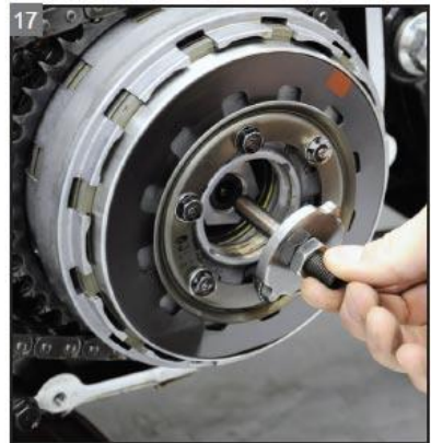
17 Remove the clutch adjuster plate.
