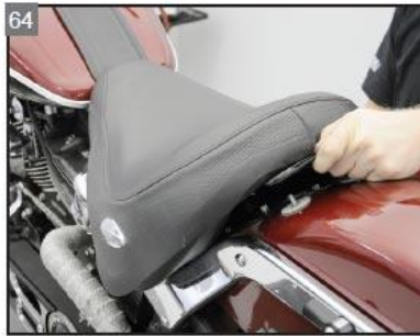
64 Install the rider and passenger seats.
