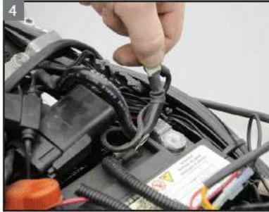
4 Move the negative battery cable away from the post to prevent accidental connection.
