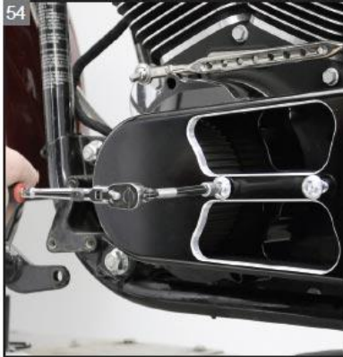
Tighten the cover's mounting hardware.
