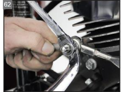
62 Tighten the linkage hardware.
