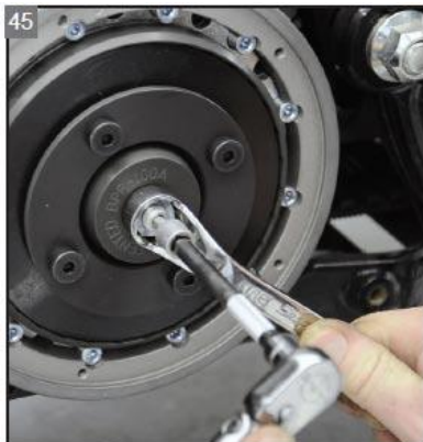
45 Tighten the clutch adjuster's locking nut.
