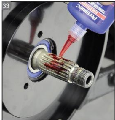
33 Apply red Threadlocker to the mainshaft splines.
