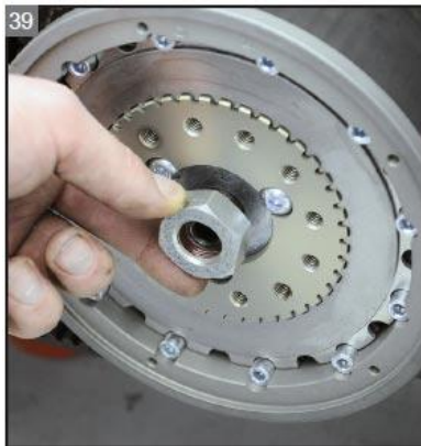
Install and tighten the clutch nut (lefthand threads).
