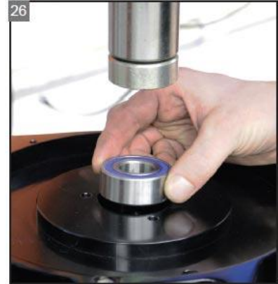
Align the sealed bearing with the BDL motor plate.
