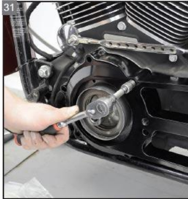
31 Install and tighten the motor plate mounting hardware.
