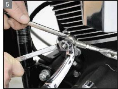
5 Loosen the shift linkage from the front shift arm.
