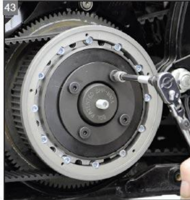
43 Evenly tighten the pressure plate hardware to the clutch hub.
