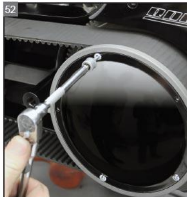
52 Install the clutch cover mounting hardware.
