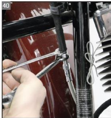
Loosen the clutch cable adjuster.
