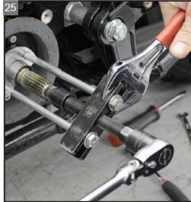
Pull the bearing race off of the mainshaft.
