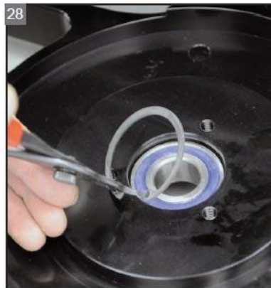
Install the bearing-retainer snap ring.
