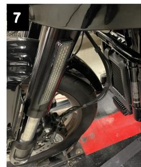
10. Plug the LRST LED fork reflectors into the LRST adapter harness at both turn signals. Use cable ties to secure wires from being cut, frayed, or pinched.
