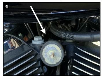
The Horn labeled with "H" is the High. The Horn Labeled with "L" is the Low. Connect the long black (-) wire and long red (+) wire of the Horn Y harness to the High tone horn terminals. The horn terminals are not polarity sensitive.
