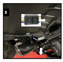
7. Remove left and right OEM front turn signals.
