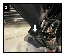
Pull outer fairing away from inner fairing and unplug headlight connector shown in **Figure 4**. Remove outer fairing and store in a safe place to prevent damage.
