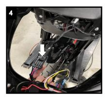
Locate left and right turn signal connectors and unplug by pressing down on the releasing tab shown in Figure 5.
