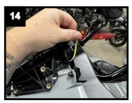
Install Center Windshield Trim LED to top vent cover by sliding the rubber posts into slots in cover all the way onto the cover. Shown in Figure 15.
