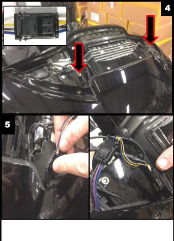
Secure and route the windshield trim harness for each side. Route the wires towards the inner fairing. You will notice a small gap at the point where the inner and outer fairing mate. This is where the wires will exit. (shown in Picture 6 and 7)
