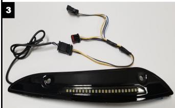
4. Connect the left and right windshield trim, with the Harness installed, inline with the left and right 3 pin JAE plug on the bike. (shown in Picture 4 and 5).
