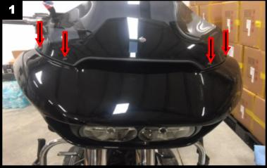
Once the windshield fasteners and windshield are removed, you will need to remove the vent. The vent is secured to the fairing by clips. Position yourself in the front of the motorcycle and lift straight up on the vent to release. (Picture 2) Store vent in a safe place to prevent damage.
