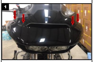
Once the windshield fasteners and windshield are removed, you will need to remove the top vent. The top vent is secured to the fairing by clips. Position yourself in the front of the motorcycle and lift straight up on the top vent to release. (Picture 2) Store the top vent in a safe place to prevent damage.
