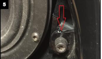
Locate and remove the lower T-25 screw on each side of the inner fairing.
