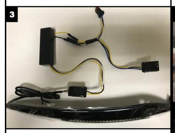
Connect the left and right windshield trim, with the A/W Convertor Harness installed, inline with the left and right 3 pin JAE plug on the bike. (shown in Picture 4 and 5).
