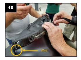
Time to re-install the fairing, make sure to plug in the H4 connector back onto the headlamp. Hold the windshield trim above the fairing, then push the outer fairing cover into place. Next put the windshield trim into position and secure loosely with the provided washer and new center 1/4-20 x 2 1/4 bolt. Make sure the wires route at the sides of the fairing as shown. Since the single bolt is loose, we are now able to reinstall the windshield, let it rest there for now.
