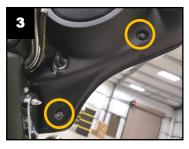
Pull the fairing away from the bike, then disconnect the H4 Connector from the headlamp. Store fairing in a safe place for reinstallation later.
