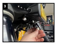
Adjust the Light Bar and tighten the M5 Allen Screws from Step 3 to secure the Light Bar in place. Shown in Figure 4.
