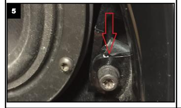
Locate and remove the lower T-25 screw on each side of the inner fairing. Refer to Photo #6
