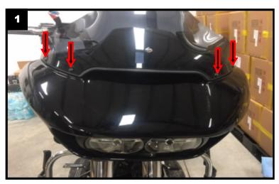
2. Once the windshield fasteners and windshield are removed, you will need to remove the top vent. The top vent is secured to the fairing by clips. Position yourself in the front of the motorcycle and lift straight up on the top vent to release. (Picture 2) Store the top vent in a safe place to prevent damage.
