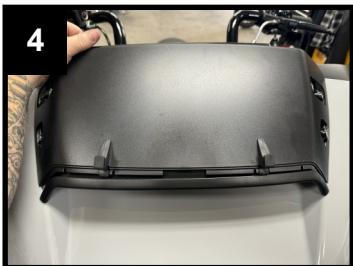
6. Remove outer fairing by removing the speaker grills that are held into place with retaining clips, pry up at the inner edge and pull away from motorcycle. Remove the 2 screws in speakers area and the 2 screws down at the fairing wind deflectors and remove the final 4 screws at the top of the fairing and remove fairing gently.
