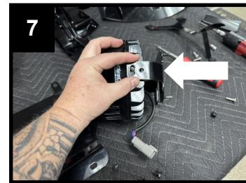
10. Install both Shark Demon® 2 LED Headlights and SD-HL Bracket assemblies to the Main Headlight Bracket using the supplied M6 Serrated Nuts. Shown in **Figure 8**.
