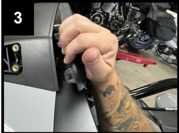
5. Remove vent cover by lifting up and out and do not lose the rubber windshield posts. Shown in **Figure 4**.
