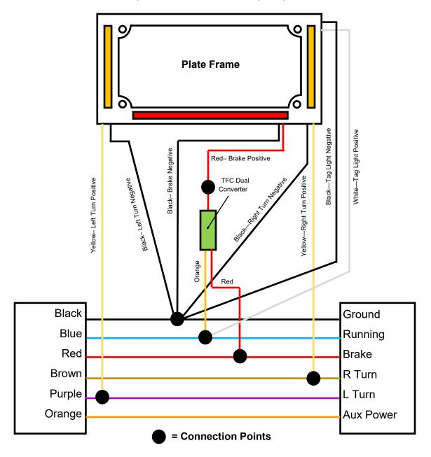
Diagram depicts the wiring color codes for a typical Harley-Davidson wire harness, when installing on other makes, please refer to your owners manual or service manual for the appropriate wire color codes. Use a meter and or test light to determine wire function if the former is not available. Not for use with bikes without a center tail light. If using with a Run Brake Turn Controller, the product must be installed before the RBT signal for correct operation.
