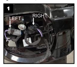
Connect the Integrated LRST Taillight Turn Signal Adapter
