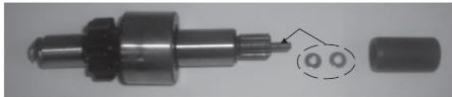
Fig-2 (If gap is too large, use shim inserts)
