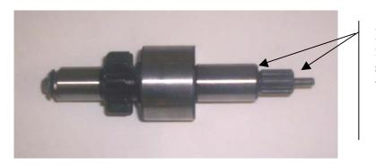
Remove material from these two surfaces as required to meet air gap of .075" - .125"
