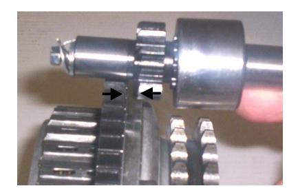
**Fig-1** (Adjust air Gap to .075" - .125")
