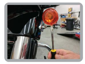
3. Push in and turn bulb counterclockwise to remove. Stock lens and bulb will not be reused.
