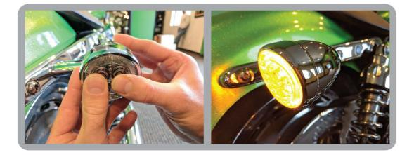
6. Turn on ignition and check for proper turn signal function.
