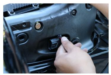
**8.** Route wires to the back of each saddle bag and secure with zip ties and brackets provided in the package. Ensure that you leave enough space between the bag lid and the mounting of the zip tie brackets.
