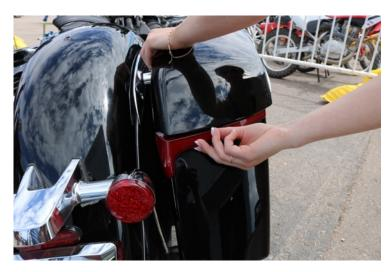
**5.** Install the lights by removing the adhesive protection strips. Be careful! Once these lights are placed and pressed on, it will take an act of congress to make adjustments to the light.
