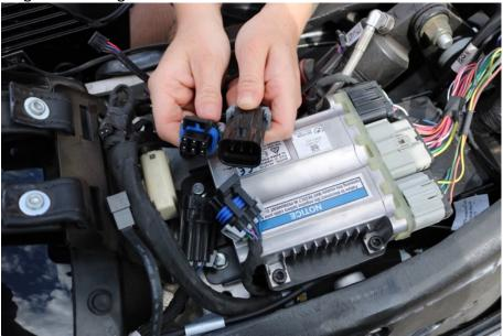
7. Route the wires from the wiring harness. The wires are long enough to enable you to route the ends through to the other accessory plug area on the frame of the bike on either side. This makes it so that you can quickly disconnect the lights if you're taking the saddlebags off.
