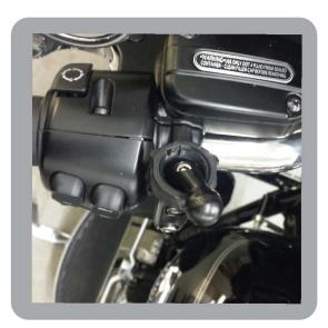
2. Snap your drink holder onto the ball and thread the large plastic nut back onto the drink holder. Adjust the angle, tighten it down, and you are ready to go.
