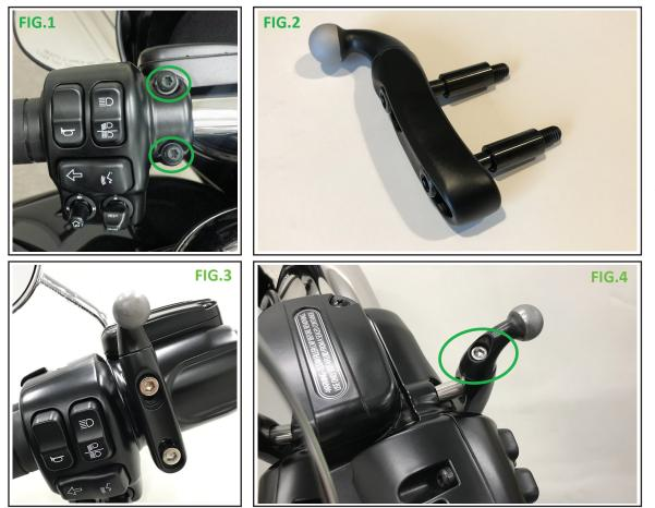
3. Compare the screws you removed to the screws included in this kit. Both 1/4-20 and M6x1.00 threaded screws are included to cover a variety of applications. Use the screws that match your motorcycle. Prepare the perch mount as shown above. (Fig. 2)
