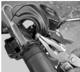
Figure 3; remove cables and brass ferrules from grip.
