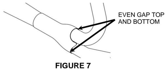
25. Once the collector heatshield is aligned properly snug the clamp but **DO NOT TIGHTEN** at this time.
