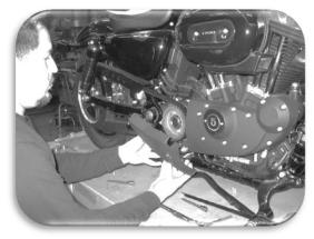
STEP 5 MOVE BRAKE ROD AND PEDAL ASSEMBLY
