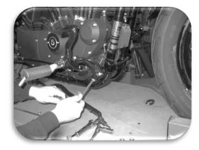
STEP 7 REMOVE FACTORY EXHAUST BRACKET
