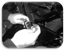
STEP 2 DISCONNECT FRONT AND REAR O2 SENSOR
