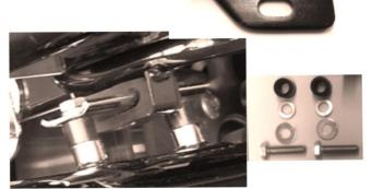
Muffler Bolts and Spacers W 1/2 OD Round 5/8 ID 3/8 5/16-18 x 1 1/4 Hex Bolt, Flat Washer, Lock Washer ■
