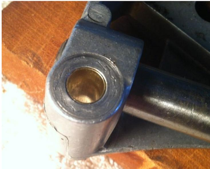
**3B. Bike Installation:** For installation on the bike, you do not have to remove the plate, but it needs to be loose so that the Rocker Lockers can center the plate when it is tightened, it also takes the pressure off the shaft so that it can turn/get the notch lined up, and let the Rocker Locker pull past.
