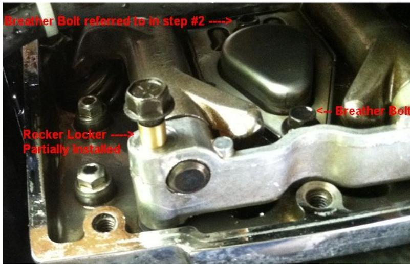
Pull a bolt out of the right side of the plate, (facing forward on the bike) this is the side that locks the shaft. Insert the Rocker Locker in the hole; they are tapered, put the small end in the hole.
