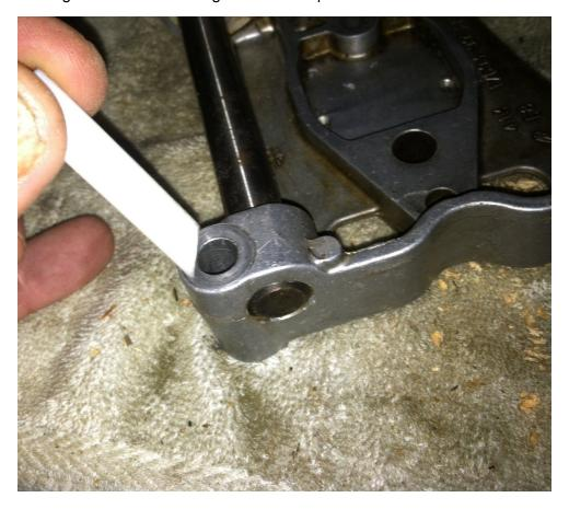
The Rocker Locker ready to be pressed into the Rocker Cover Inner by the bolt, washer, and nut set-up.
