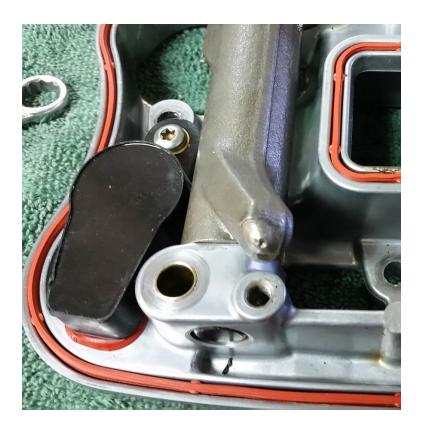
**4.** Before bolting the Rocker Cover Inner in place, use some q-tips to clean out the bolt holes in the head (compressed air will also work, but might be a bit messier than q-tips, if you use compressed air protect your eyes). You want to get rid of any debris and any oil that may be in the threads. Install/torque your Rocker Cover Inner & Rocker Cover according to your Service Manual instructions & specs.
