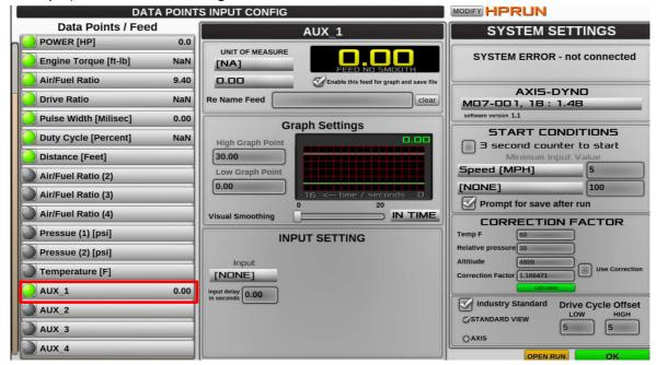
3. Re name the feed if needed and select the input channel according to the chart above (Belt Temperature and AIN00 in this example)
