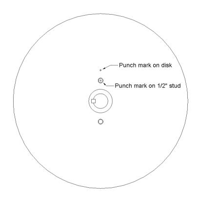
The punch mark on the ½" stud needs to be aligned with the punch mark on each disk and oriented vertically before tightening
