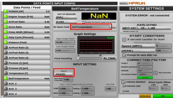
4. Set the inputs delay if needed and the calibration variables for the particular sensor (In this example, 0.25 volts = 32 F and 4.75 volts = 212 F)
