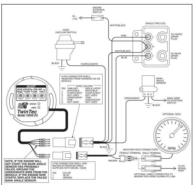
Figure 4 - Single Fire Wiring Diagram
