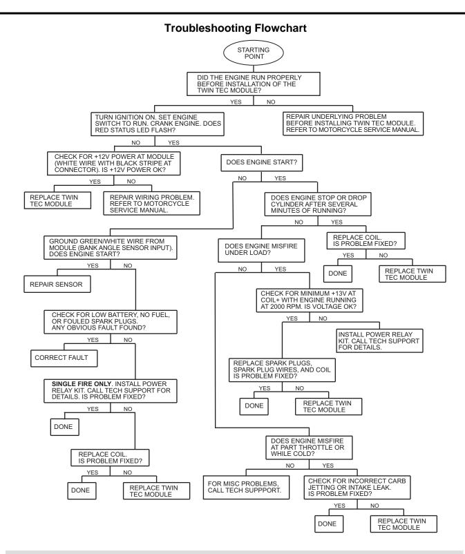
TROUBLESHOOTING TIP: If you are installing an internal (nose cone) ignition for the first time and the engine will not start, the most likely problem is improper static timing. Make sure that the front piston is at TDC on the compression stroke and not on the exhaust stroke. Also check the bank angle sensor as described above.
