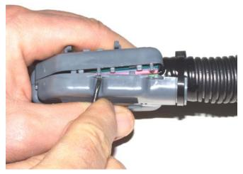
Figure 4 – ECM Connector Terminal Removal
