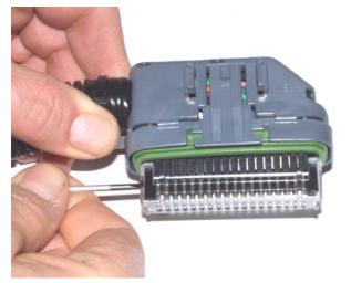
Figure 3 – ECM Connector Disassembly
