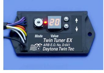
You can use the mode and up/down pushbutton switches to make fuel trim adjustments in the RPM and throttle position ranges required by most applications. The fuel trim value is displayed on a bright daylight readable LED display.
