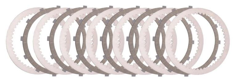
This kit consists of 6 friction and 7 steel plates. Plates should be pre-soaked in the same fluid you will be using in the bike for about 10-15 minutes. The type of fluids we recommend are any HD petroleum based, non-synthetic, primary oil, as light weight as possible, or even a good petroleum based motor oil such as 10/40 or 20/50 in weight. You can even use ATF Type F or B&M Trickshift. THE USE OF SYNTHETICS IS NOT RECOMMENDED AS THEY TEND TO CAUSE SLIPPAGE.
