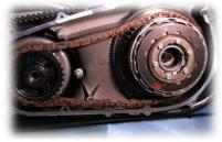
4) Install new 30 Tooth sprocket chain and basket. Figure 5
