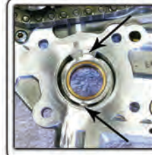
Inspect camplate for scoring, if scoring is present replace camplate. Scoring will effect oil psi & oil scavenging
