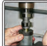
Press cam gears onto camshafts
