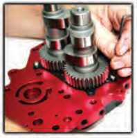
Install bearing retainer plate using loctite
