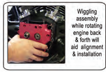
Install camplate & oil pump as a complete assembly
