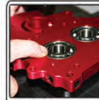
Verify bearings are flush with camplate
