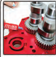
Install bearing retainer plate using loctite
