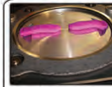
clay pistons and measure thickness of clay after cycling engine
