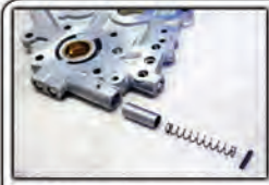
Inspect pressure relief valve
