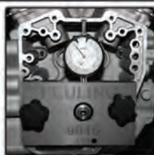
Feuling Runout Measuring Tool #9015
