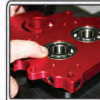
Verify bearings are flush with camplate
