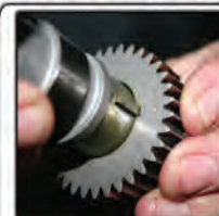
Line up gear with camshaft
