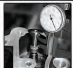
Installed valve spring height is critical!
