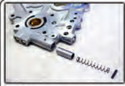
Inspect pressure relief valve
