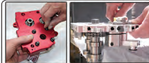
Bolt oil pump to camplate finger tight DO NOT use loctite or hardening compound
