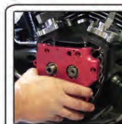
Wiggling assembly while rotating engine back & forth will aid alignment & installation
