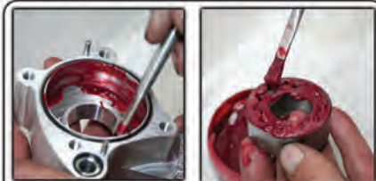
Apply engine assembly lube to oil pump housings & gears
