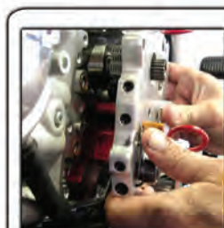
Install camplate & oil pump as a complete assembly
