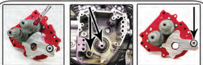
Apply engine assembly lube to camshafts, inner cam bearings, scavenge port hole of case and pick up port of oil pump
