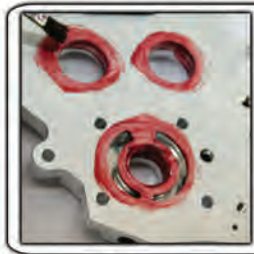
Pre-Lube camshaft bores, thrust surfaces, Pinion bore and oil pump mounting surface
