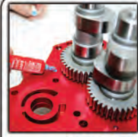
Install bearing retainer plate using loctite
