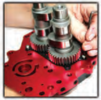
Install bearing retainer plate using loctite
