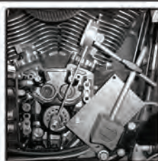
Dial indicator with Magnetic base
