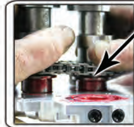
When installing camshafts into the late model camplate lead with the rear cam
