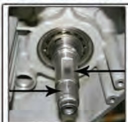
Remove burrs & scoring from pinion shaft to assure smoothness
