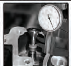
Installed valve spring height is critical!
