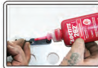
Apply Loctite to block off plate bolts
