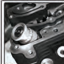
Installed valve spring height is critical!
