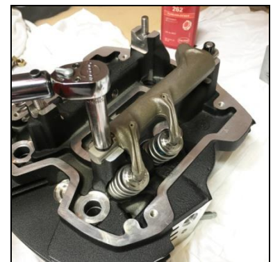
Evenly seat rocker arm to 10 Ft. Lbs loosen to allow shaft to settle then evenly step torque to final spec of 24-26 Ft. Lbs
