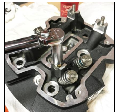
Torque stud to 4-5 Ft. Lbs
