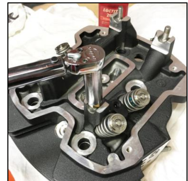
Torque stud to 5 Ft. Lbs
