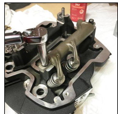
Evenly seat rocker arm to 10 Ft. Lbs loosen to allow shaft to settle then evenly step torque to final spec of 24 Ft. Lbs
