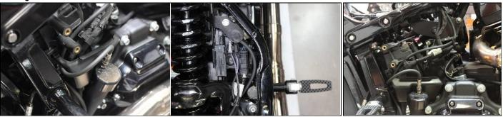
**4.)** The oil separator inserts into the inner dipstick housing bore, alternating the 3/4" OD perforated screens and spacers then the large perf screen, filter, aluminum perforated disc then umbrella valve. The smaller diameter spacer is the  $2^{nd}$  from bottom, the umbrella valve sits on top.
