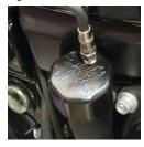
Route the breather line up under the seat, looping to follow the side cover profile hiding on the inside of frame rail, up under the seat then back down along the right side frame rail, follow inside the right frame rail and the filter element can fit cleanly between the engine/trans matting area on the inside of the lower right frame rail. Use zip ties to fasten the line and element to your frame rail.
