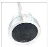
**5.)** Screw the cap on using a dab of the 545 Loctite on the threads, this will prevent leaking.
