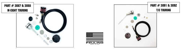
The Feuling billet dipsticks vent/breath excessive crank case pressure from the oil tank through a PVC style breather consisting of an oil separator system, perforated disc, replaceable filter element and umbrella flapper valve. Feuling vented dipsticks screw into the factory oil fill spout as a stock replacement part.
