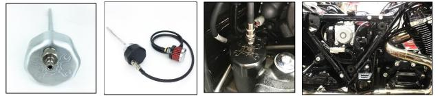
4.) Screw the cap on using a dab of the 545 Loctite on the threads, this will prevent leaking.
