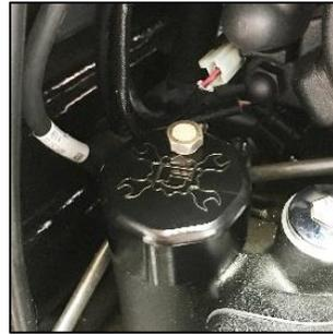
**OPTION 2.)** Quick disconnect fitting with rubber hose and filter element. This option will run any excessive oil misting/residue through the line and into the filter element. However this option does require disconnecting the fitting in order to check the oil.
