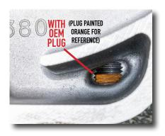
NOTE: The M-EIGHT main sump cross port on the inside of the M-Eight engine case is in a slightly different location & height in each engine case. This cross port is created when the bottom plug hole is machined and tapped by the factory. The machining breaks through the casting wall, creating the sump port. Whereas the Twin Cam engine cross scavenge pick up hole is a machined bore, and is in the same location in every engine case.
