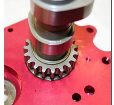
\*Always install new matching bearing race onto rear camshaft
