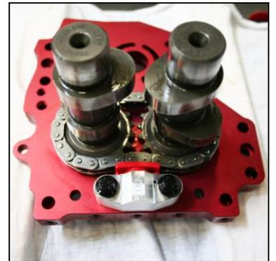
Inner cam chain + tensioners installed into '07-'16 camplate
