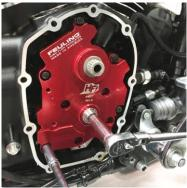
10. With the oil pump and camplate bolts finger tight rotate the engine over by hand, tighten and torque the camplate bolts first then the oil pump bolts, this process will center the camplate and pump as best as possible to the engine and crankshaft runout. Alternately step torque camplate and oil pump bolts up to a final 120 inch pounds.
