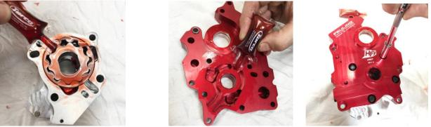
8. Rotate oil pump gears so gear flats are vertical to match the crankshaft per step 6. We found having the crank and gear flats vertical make for the easiest install of the oil pump and camplate assembly.
