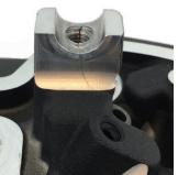
\*FEULING Rocker Stud/Nut kit #3047 will reduce stress on the rocker arm head stand offs. The rocker arm 'stand offs' are a weak link and prone to cracking.
