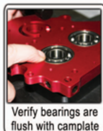
Press in camshafts use lube & proper tools
