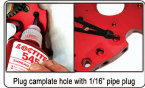
*Plug this camplate hole if case does not have a boss
