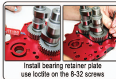
Press in camshafts use lube & proper tools
