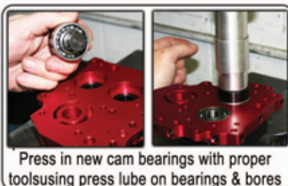
Verify bearings are flush with camplate
