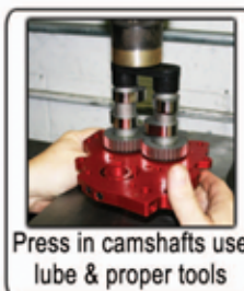
Verify bearings are flush with camplate
