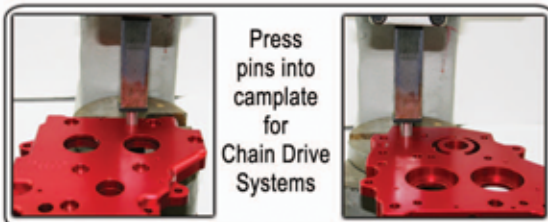
Camplate #8010 Install guide tower on camplate for Chain Drive Systems
