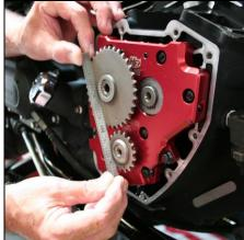
Align sprockets using a straight edge to verify correct spacer behind rear cam sprocket.
