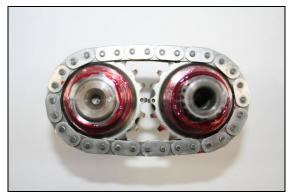
'07-'16 + conversion camshafts, inner cam chain #8060 installed with camshaft timing marks aligned. Lead with rear cam when installing into camplate
