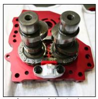
Inner cam chain + tensioners installed into '07-'16 camplate
