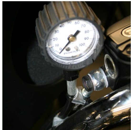
Gauge mounting next to master cylinder
