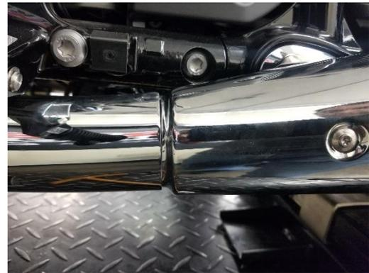
Fig 2.18 about 1/8" gap or 3mm
