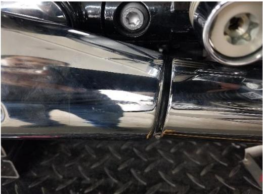
Fig 2.21 about 1/8" gap or 3mm
