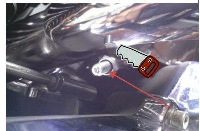
Fig 1.9 tighten T-bolt clamp and if you wish cut the end of the bolt threads flush with the nut
