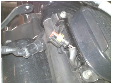
Fig 1.7 connects front O2 sensor harness and place plastic cover back in place.
