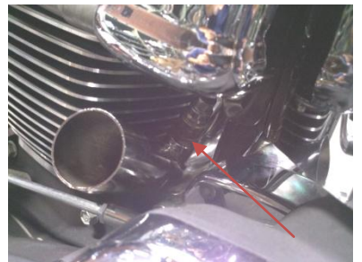
Fig 1.4 attach pipe assembly to bracket with 3/8 x 3/4 carriage bolts
