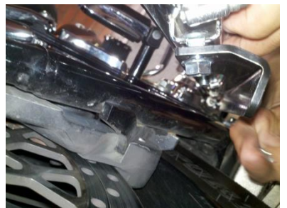
Fig 1.4 attach pipe assembly to bracket with 3/8 x 3/4 carriage bolts
