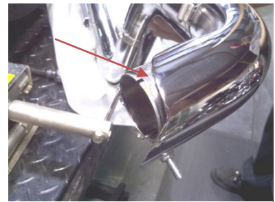
Fig 1.8 install clamp as shown on left side pipe bolt must face towards the engine to be able to be tighten
