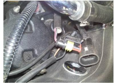
Fig 1.6 connect O2 sensor harness underneath the oil tank make sure cable is away from headers to avoid heat damage
