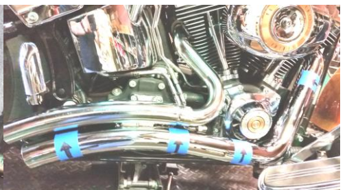
Figure 2.12 install front heat shield first and secure it with hose clamps.
