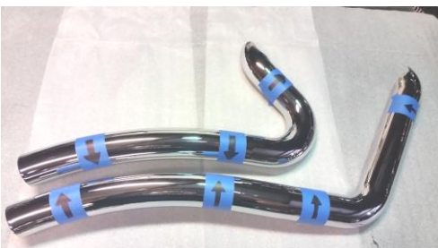
Figure 2.10 mark center and direction
