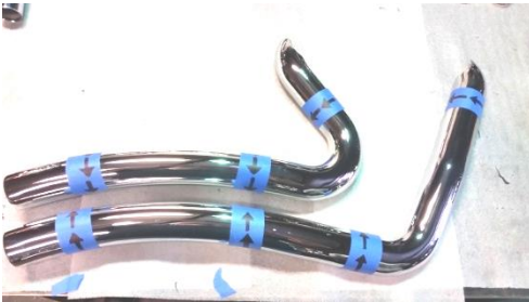
Fig. 2.7 Arrows indicate direction of hose clamp insertion
