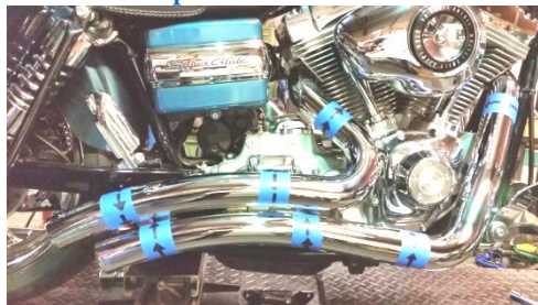
Fig. 2.7 Arrows indicate direction of hose clamp insertion
