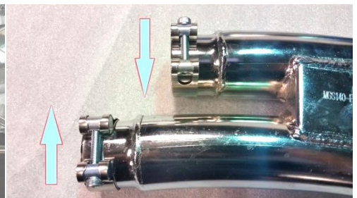
Fig. 2.3 Insert barrel band clamps over the muffler inlets as shown
