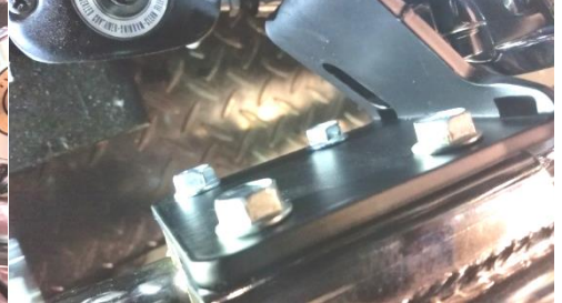
Fig. 2.6 bracket shown with muffler attached to it.
