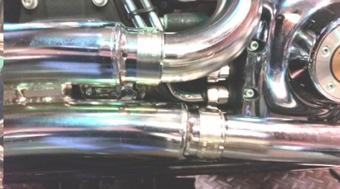
Fig. 2.5 Install muffler as shown
