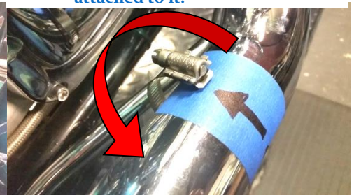
Fig.2.9 Hose clamp insertion sample
